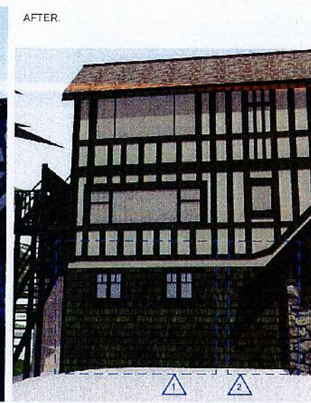
RENDERING SHOWING STAIR AND WINDOW REMOVED AND PROPOSED 30" SQUARE WINDOWS.
