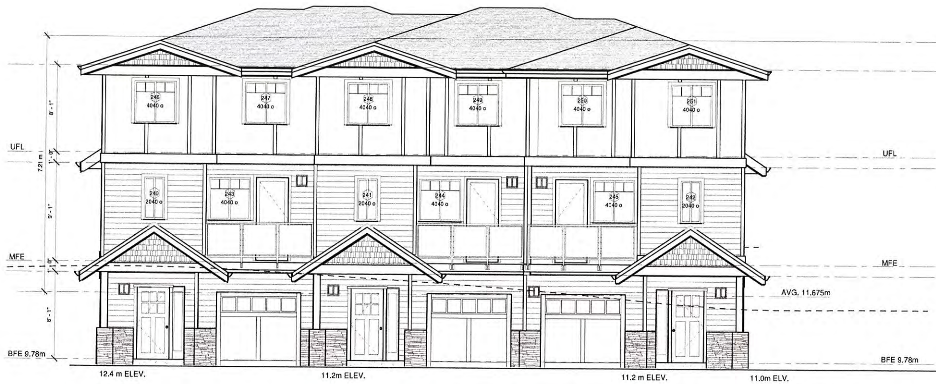
1 Front (East) Elevation 1/4" = 1'-0"
