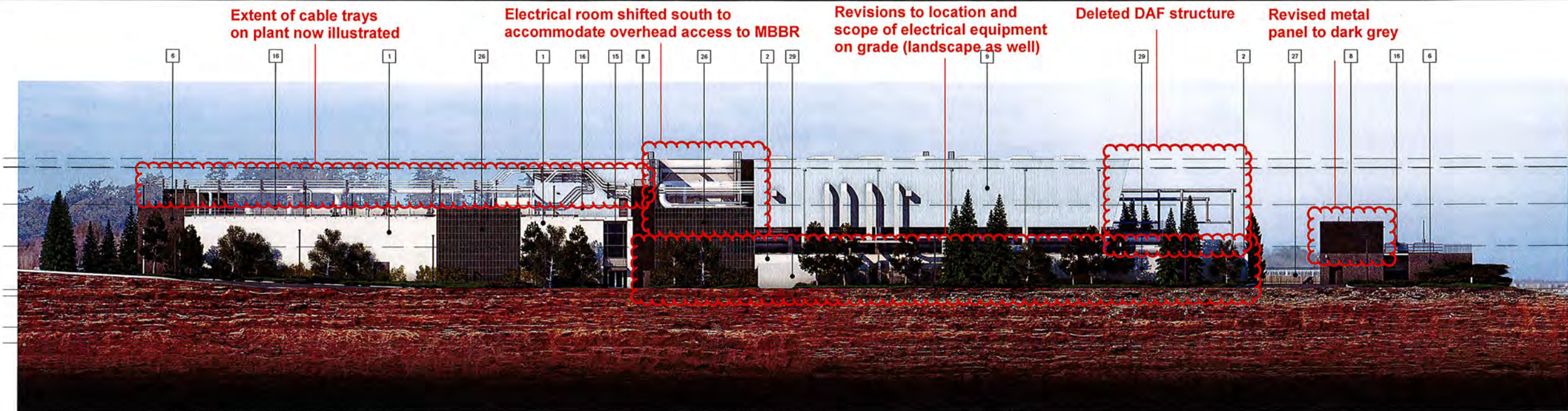
1 BUILDING ELEVATION - WEST B5-DP-A-7 SCALE: 1:250
