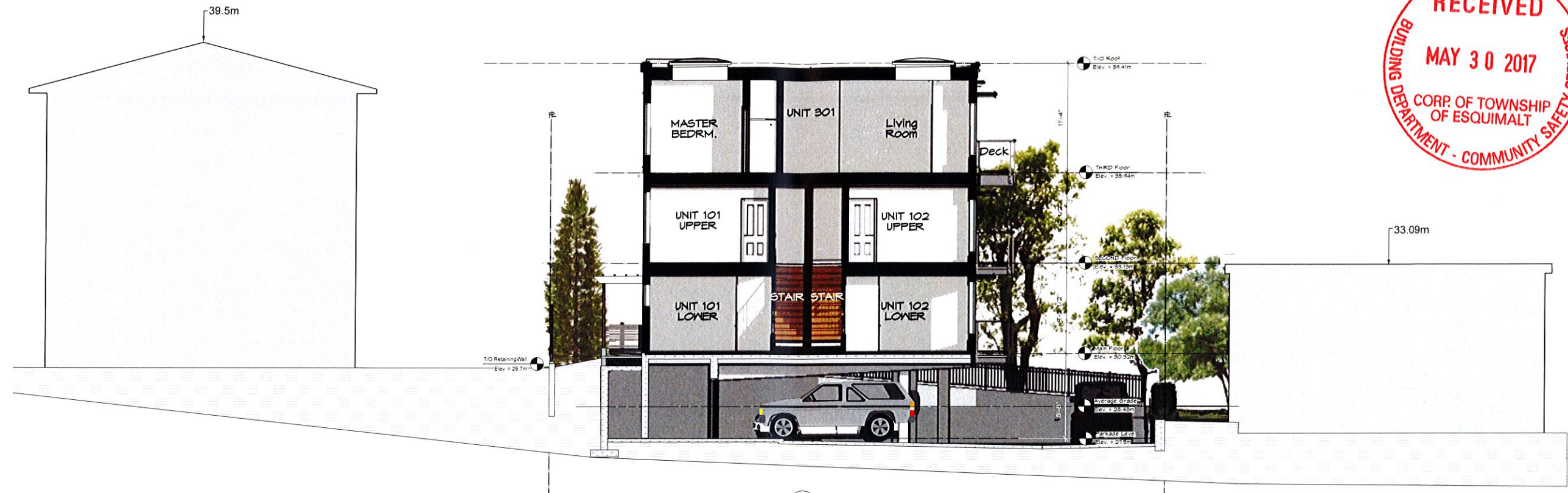
2 North/South Section Looking East Scale: 3/16" = 1'-0"
