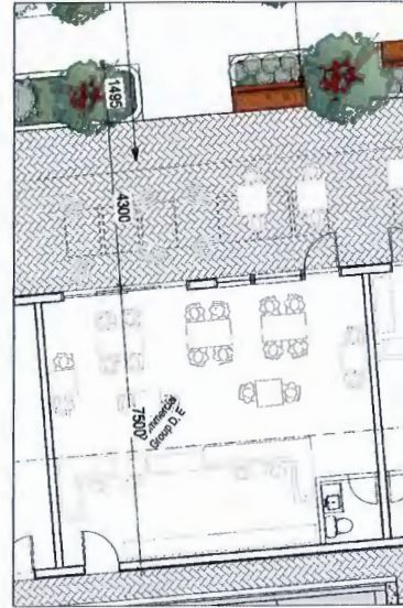
Suite CRU3 Commercial suite 59.5 m 2 inside GWB / 62.9m 2 to cl walls / 677 R2 Group D, Group E Parking 59.5m 2 @ 25m 2 /st = 2.38
