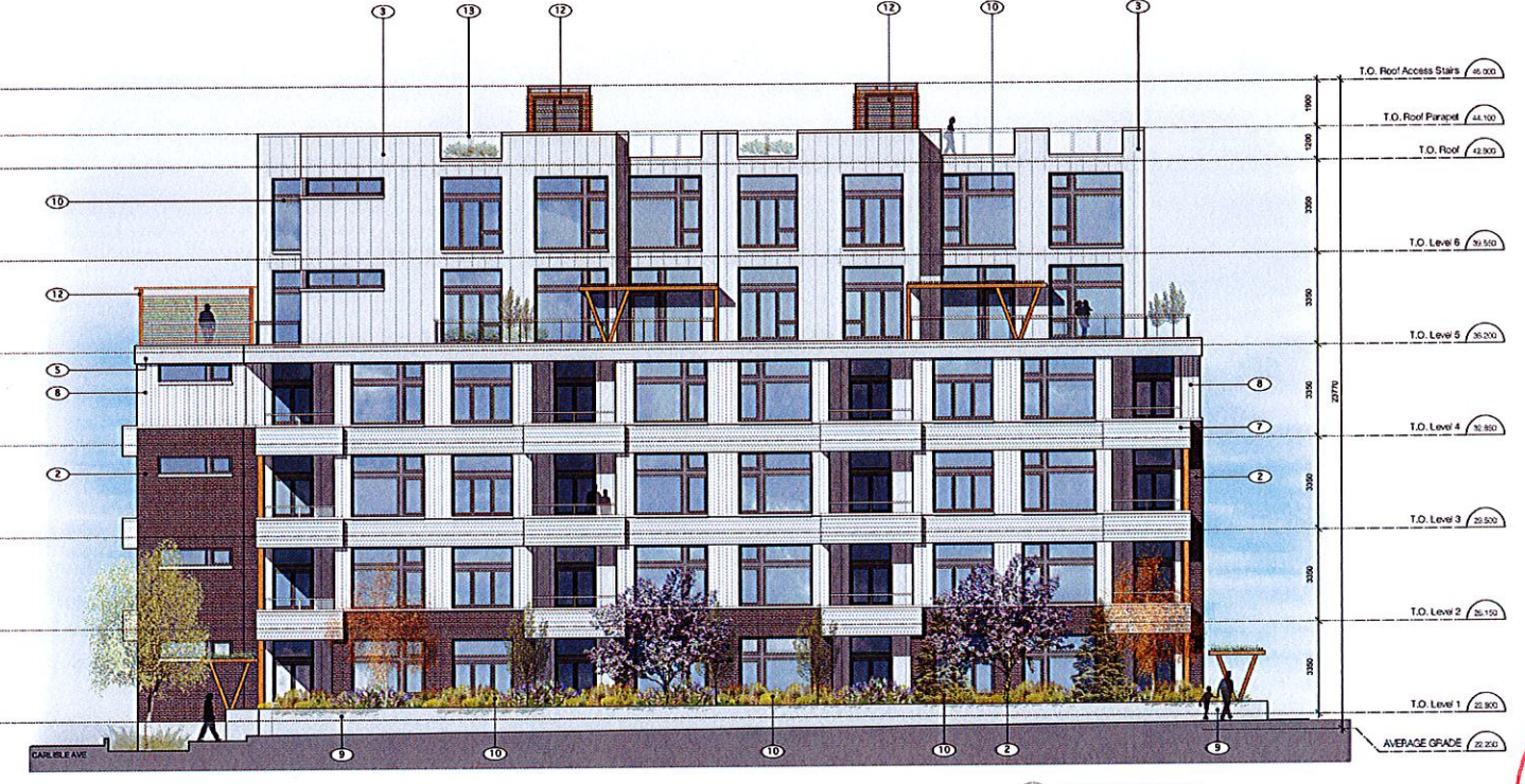
2 Elevation East (Bldg B) Scale: 1:100
