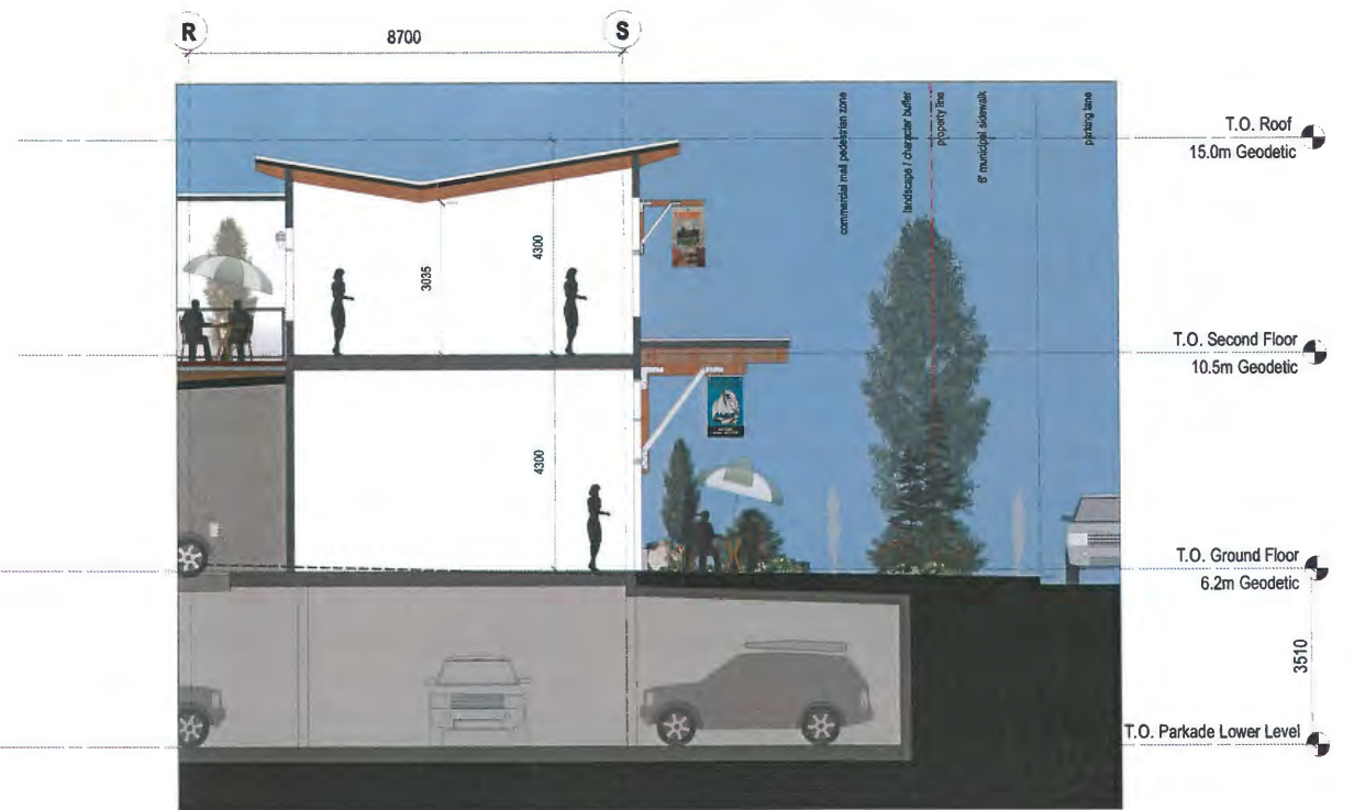
4 Building 1 - Detail Section A4.3 Scale 1:75
