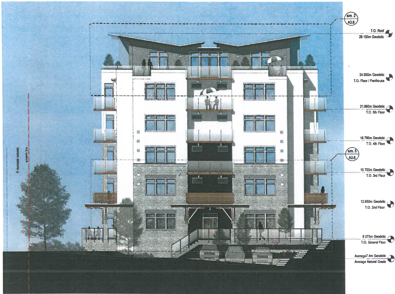
1 Building 2 - [east] Exterior Elevation A3.10 Scale: 1:100
