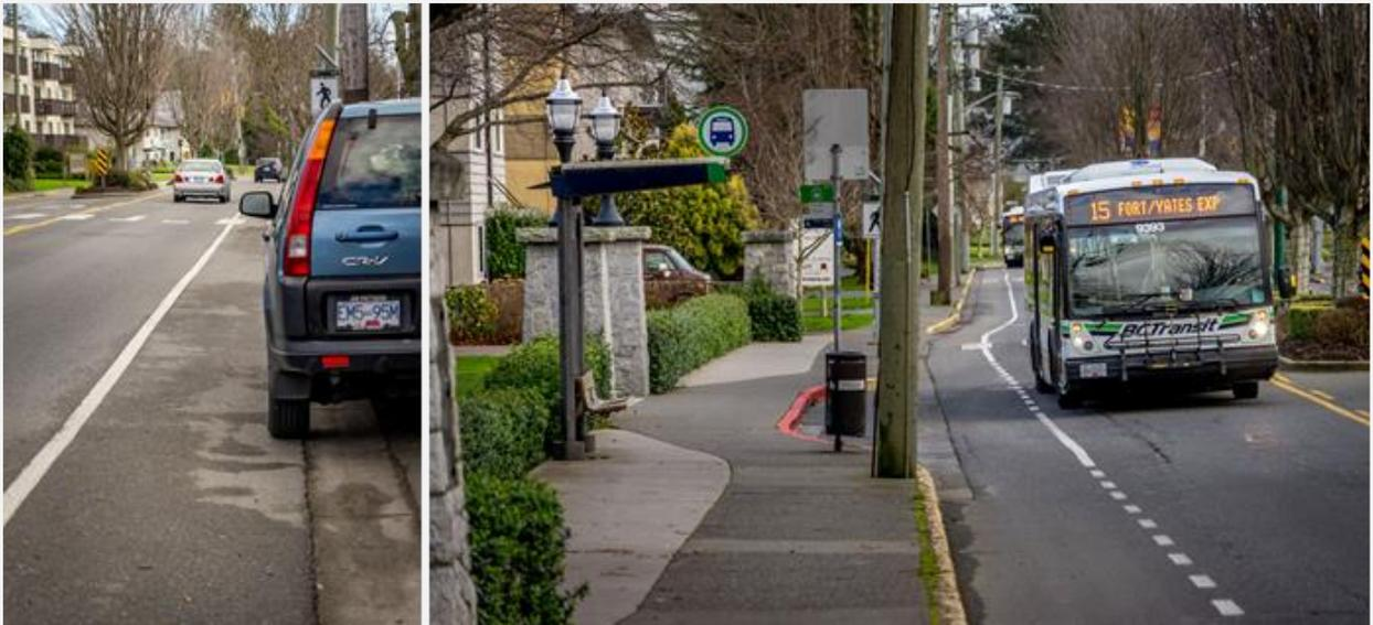
*The combination of on-street parking, medians, and bus layovers make it more challenging to provide a cycling facility with full protection for all sections of the Esquimalt Road corridor.*
