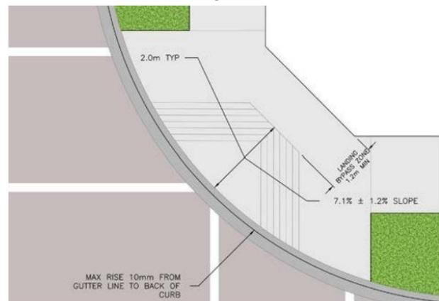
Example of a combined curb ramp. They allow people using wheelchairs to enter the crosswalk along a straight trajectory, unlike a single curb ramp that is located at an angle to the road.
