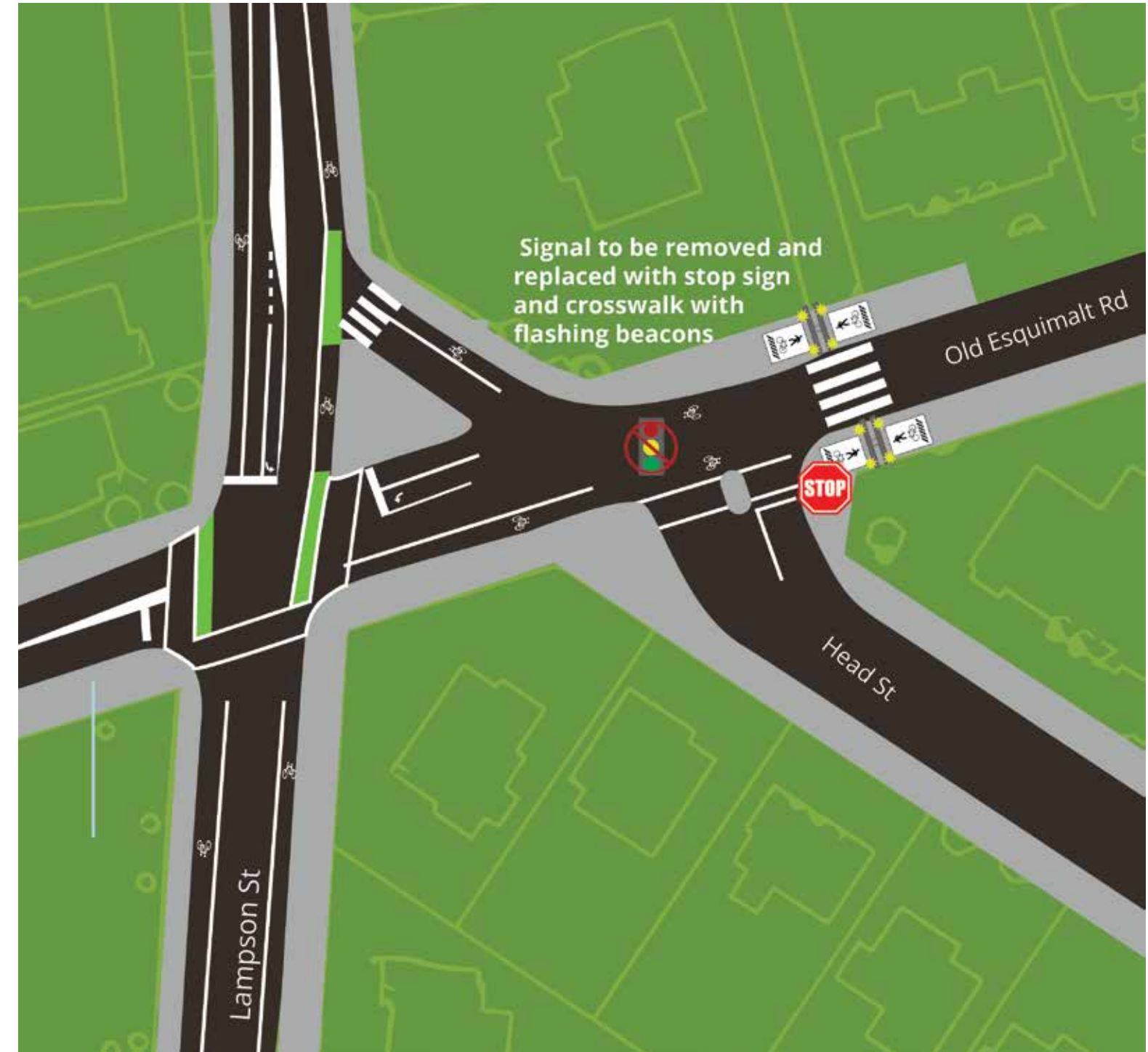
IMAGE: REPLACEMENT OF TRAFFIC LIGHT WITH CROSSWALK AND FLASHING BEACONS
