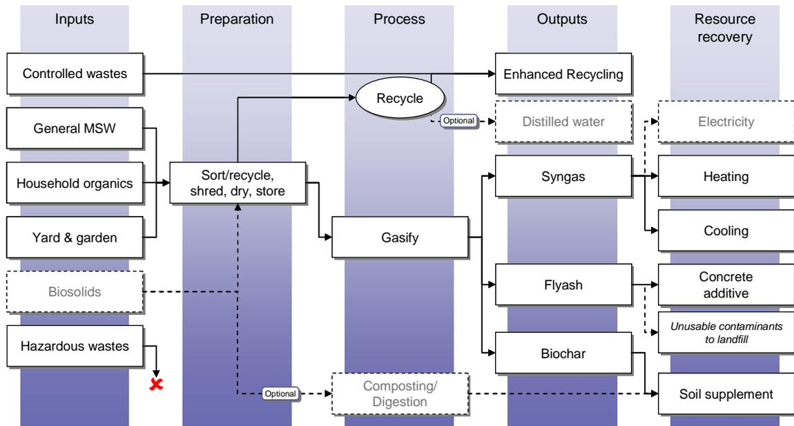
Figure 28: Gasification General Process
