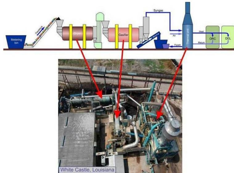
Figure 48: Schematic Overlay of White Castle Plant
