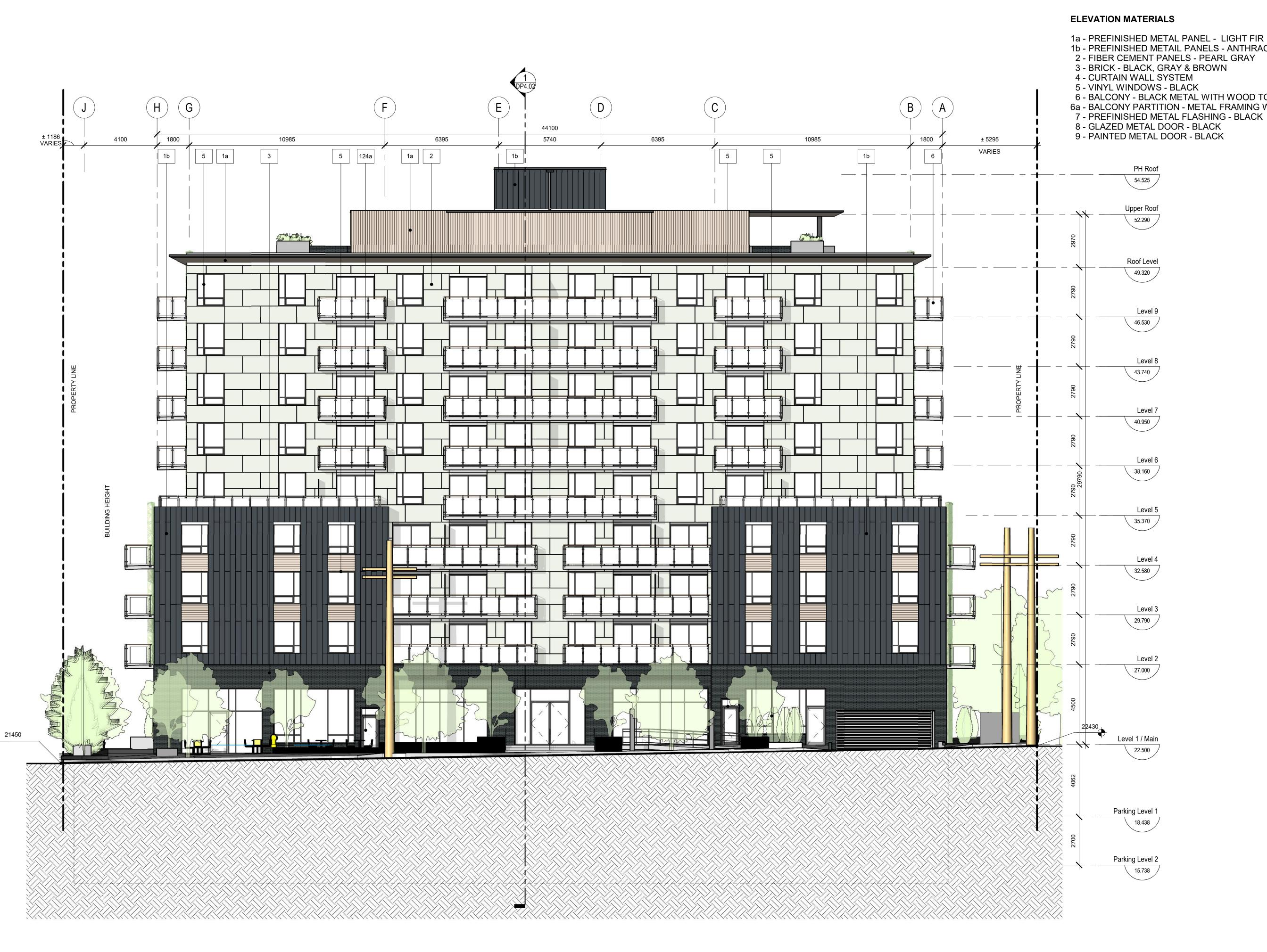
1b - PREFINISHED METAIL PANELS - ANTHRACITE GREY 6 - BALCONY - BLACK METAL WITH WOOD TOP RAIL 6a - BALCONY PARTITION - METAL FRAMING WITH FROSTED GLASS
