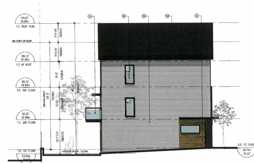
6 BUILDING B - WEST ELEVATION (SIDE) A201 NTS
