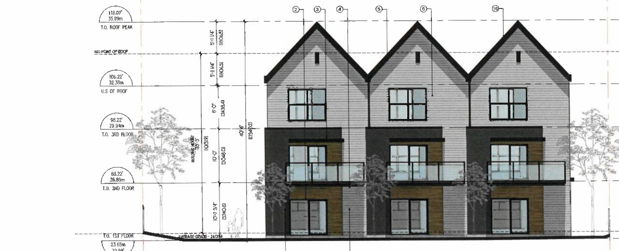
5 BUILDING B - SOUTH ELEVATION (REAR) 1/8"=1'-0"
