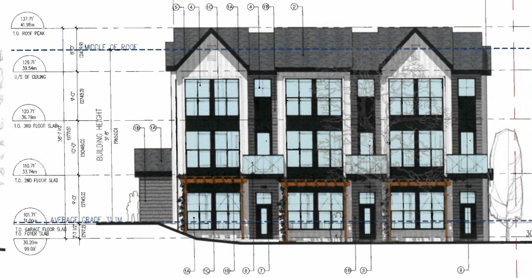
5 BUILDING A - EAST ELEVATION (FRONT)
