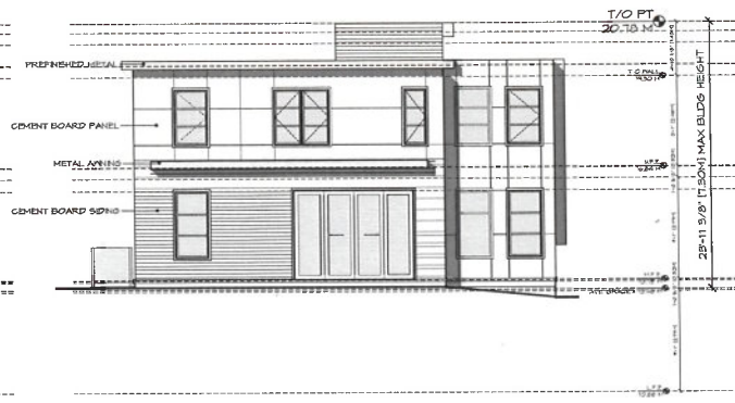
6 Rear Elevation (Lot B) DP3 Scale 1:100
