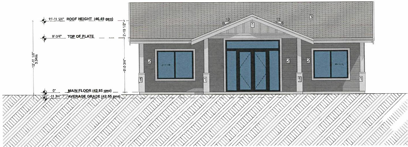
1 FRONT ELEVATION SCALE: 1/4" = 1'-0"
