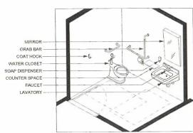
Resist a 1.3 kN load vertically and horizontally (not simutaneo
