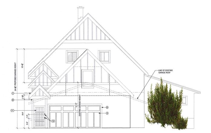
FRONT ELEVATION WITH NEW BREEZEWAY Scale: 1/4" = 1'-0"
