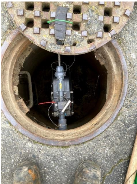
Figure 7-2: Echo Level Logger Setup
