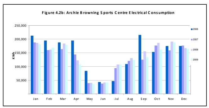
In Figure 4.2 b, above we notice that the monthly electrical consumption is also seasonal with the compressors and brine pump shut down for some of April, May, June and some of July. When we look at the monthly consumption trend, it appears that the monthly consumption is peaked at around 185,000 kWh per month.
