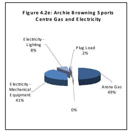
In Figure 4.2 e the overall energy consumption chart shows our estimate of the energy consumption breakdown associated with electrical usage and building gas heating usage. We see that the estimated natural gas usage accounts for 49% of the energy consumption for this facility, so this will be a focus for our study.
