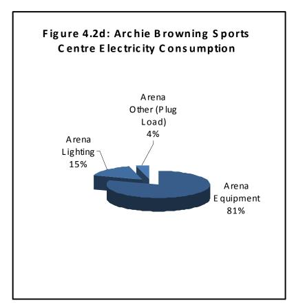
Figure 4.2d. we have analyzed the breakdown of energy consumption by building system in order to estimate the percentage of load each system represents. In this figure we see that the lighting and the arena mechanical loads make up the majority of the electrical consumption.
